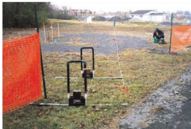
Figure 2 | GPR can be used to detect leaks in water pipes by detecting anomalies created by leaking water in the pipe depth (Hunaidi 1998) thermal infrared imaging.
