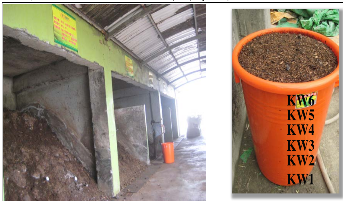
Fig.3 Counter current plug flow reactor of field study
